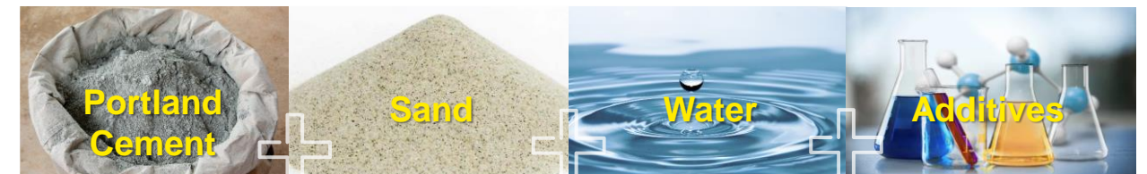
Modification of basic materials: Cement (Binder) & Sand (Filler) with chemical additive for improved chemical and physical properties
