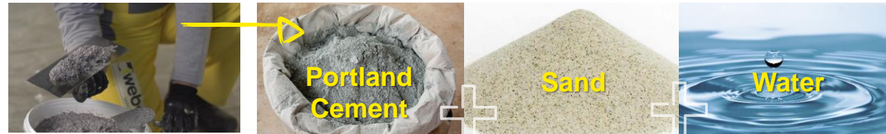
Use Cement-Sand Mortar (cement shrinkage during curing)
