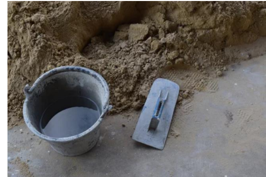
Mortar gauged with water – Limited scope of application
